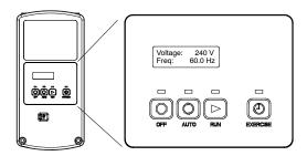
The DC2 controller provides integrated control for the generator set, Kohler® Model RXT transfer switch, programmable interface module (PIM).
